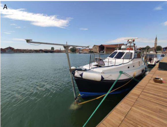
Kongsberg EM2040DC Multibeam echosounder system (MBES)
