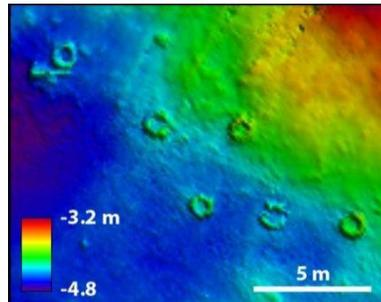
**Figure 1 Example of tires on the Venice Lagoon seafloor mapped with a high resolution MBES (modified from Madricardo et al., 2019).**
