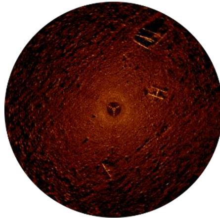
**Figure 4 Tegnù Cavallino Vicina. Example of a seafloor image obtained with the HRSS -MS 1000 that shows the presence of metallic structures of ghost nets (from Fiorin et al. 2014b).**
