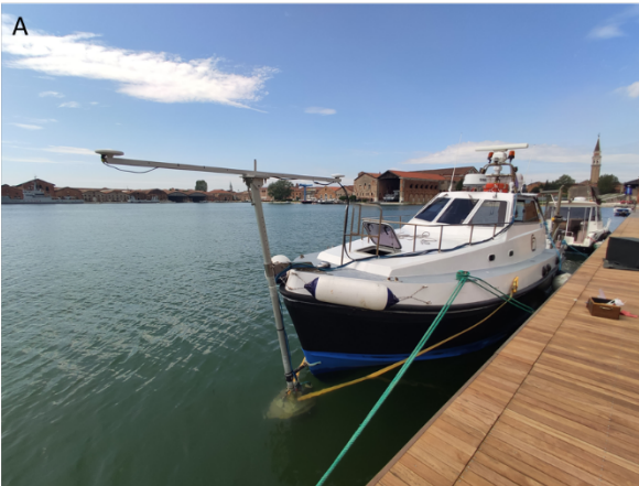
Kongsberg EM2040DC Multibeam echosounder system (MBES)
